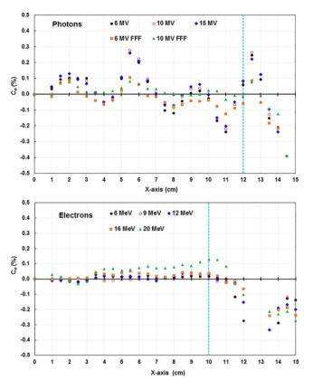
**Fig. 2.** The calibration uncertainty  $C_{\sigma}$  of the detectors in the x-axis. Data acquired at SSD = 100 cm, 30  $\times$  30 cm<sup>2</sup> field, and 2 cm solid water buildup for photons, and a 25  $\times$  25 cm<sup>2</sup> cone without buildup for electrons. The vertical blue dashed lines indicated the positions of 80% of field size.
