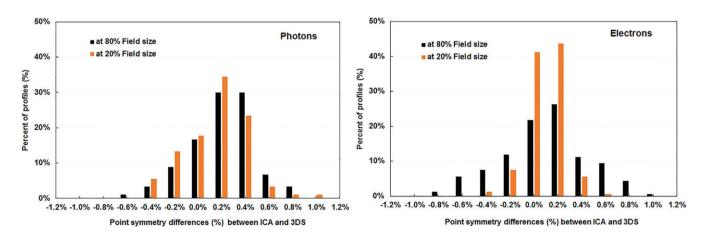
FIG. 6. Histogram distributions of the differences of point symmetry measured with the ICA and 3DS at the off-axis positions of 20% and 80% of field size for photon and electron beams. All beams were steered with the ICA. Differences in point symmetry are defined by Eq. (5).
