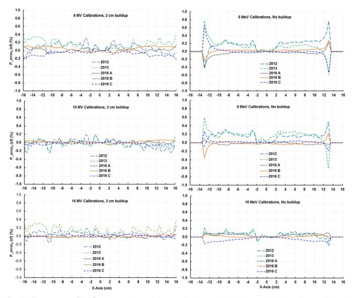
**Fig. 1.** The percent errors [Eq. (2)] of detectors along *x*-axis for array calibrations performed in the same day in 2016 and in years 2012 and 2013. Only the *x*-axis is presented but all four axes showed similar behavior.
