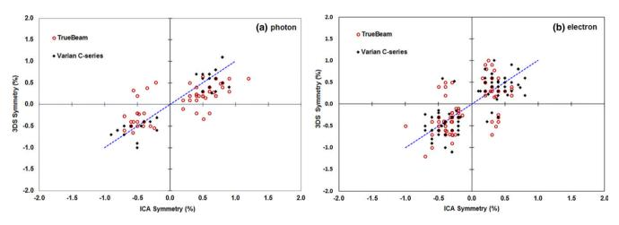
**FIG. 8.** A comparison of symmetry measured with the ICA vs. that measured with the 3DS. The symmetry was recalculated in Excel to provide an identical symmetry metric between the ICA and 3DS systems. We separated the results from Varian C-series (black) and TrueBeam (red), and found that results do not depend on the type of machine.
