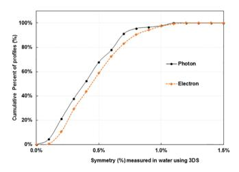
**FIG. 4.** The cumulative distributions of photon beam symmetry and electron beam symmetry measured in water with the 3DS after the beams were steered with the ICA. These data represent 90 photon and 160 electron beam profiles acquired on both C-series and TrueBeam machines.
