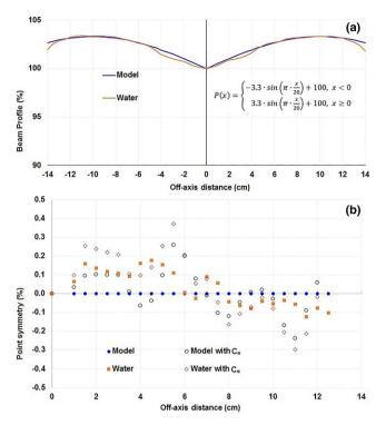
**Fig. 3.** A simulation study to show the effect of array calibration uncertainty on an idealized symmetric profile (Model) and a measured in-water profile with a 0.2% symmetry (Water) both for  $30 \times 30 \text{ cm}^2$  fields (a). Point-by-point symmetry in the central 80% of these fields is plotted both with and without applying the measured uncertainty from a 6 MV ICA calibration (b).
