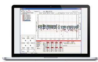
Daily QA 3 software provides a graphical presentation of data for each template. Users have the option to choose which data parameters to view and over what period to view them. A single measurement instance can be examined by clicking on a data point which corresponds to a particular measurement.
