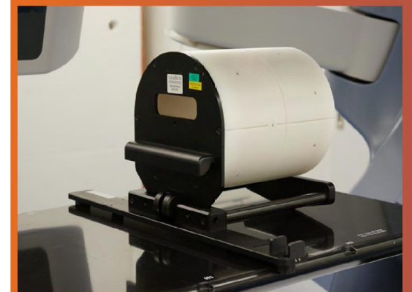
Figure 1: Isocal phantom with known geometry. Multiple MV and kV projections are acquired and automatically analyzed.
