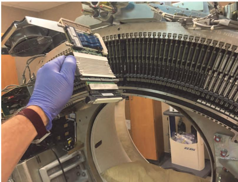
**Figure 1.15** A detector module being replaced on a 64/128 (i.e.,  $\approx 4$  cm coverage) channel CT scanner. This detector module is composed of multiple parts (scintillator, data acquisition system, analog-to-digital converter, heater) which a field engineer usually does not take apart. This particular module is in the center of the detector array and is being replaced because a ring artifact was observed that could not be calibrated away.
