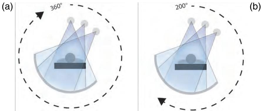
**Figure 1.10** Depiction of (a) a full scan angular range and (b) a short scan angular range. Data collection in MDCT usually uses a full scan range, but may use only a short scan range's worth of data for image reconstruction to reduce motion artifacts. CBCT systems usually can only acquire data over a short scan range.
