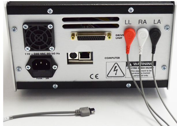
ECG signal output through snap on connections at the rear of motion controller
