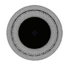
Because ArcCHECK detectors always face the delivery beam regardless of gantry angle, detection of very small gantry angle errors are possible. In contrast, when a 2D array is irradiated obliquely, the geometry collapses to 1D. Even when there is no detector shadowing effect, significant information is lost on a 2D array, and errors up to 10° are missed 75% of the time.1
