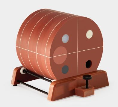
The CT ACR 464 Phantom enables comprehensive testing, including positioning and alignment accuracy, CT number accuracy, slice thickness, low contrast detectability, image resolution and uniformity, spatial resolution, and inter- and intra-plane distance measurement accuracy.
