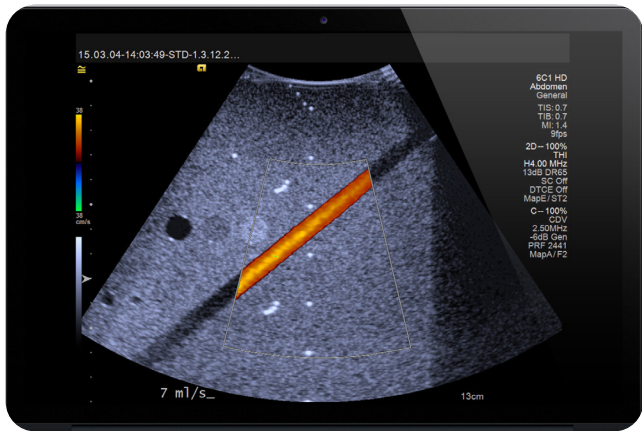
The Doppler 403 Flow Phantom is used to test the Doppler color flow velocity measurement.
