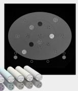
Automatically identifies phantom and location of rods.
