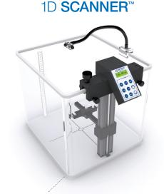
The PC Electrometer directly connects to the 1D SCANNER for monthly and annual QA.
