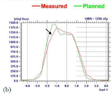
"As seen in the profile comparison, the 4.5 mm wide ion chamber detectors of the MatriXX System causes a noticeable spatial averaging effect on the measured dose."
