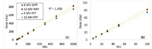
Figure 2. Dose linearities of WFF and FFF beams from 5 to 1000 MU (a). An enlarged low dose area of less than 100 MU (b).
