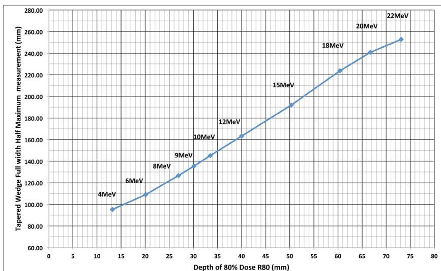
Figure 5. Depth of 80% dose vs. Full Width Half Maximum tapered wedge distance .
