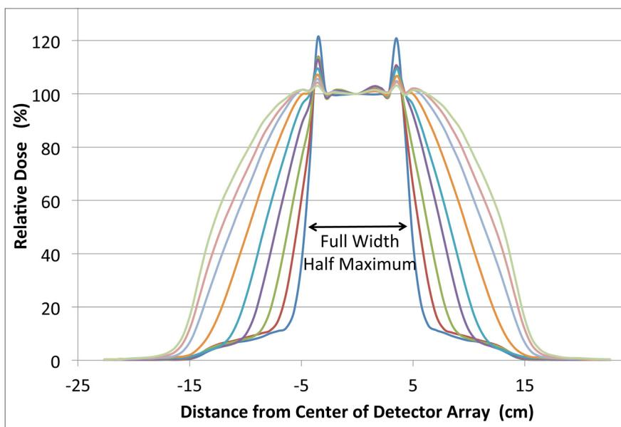
Figure 4. Profiles measured with an IC Profiler™ in combination with a pair of tapered wedges (4MeV to 22MeV electron energy) showing measurement of FWHM.
