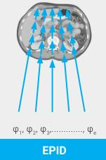
Impacts of output, MLC, Patient set-up, and Patient anatomy errors are all aliased into the fluence values  $\phi_1 \dots \phi_n$  leading to poor specificity.
