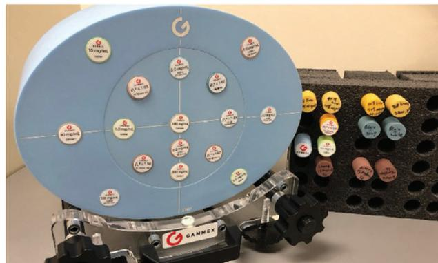
**Figure 1.** The Gammex Multi-Energy CT phantom with tissue-mimicking rods. The picture shows the “body” configuration; the central section of the phantom can be used separately as a “head” phantom.
