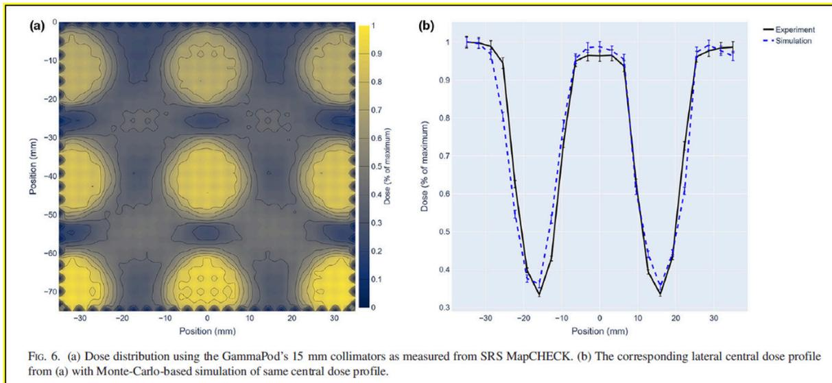
FIG. 6. (a) Dose distribution using the GammaPod's 15 mm collimators as measured from SRS MapCHECK. (b) The corresponding lateral central dose profile from (a) with Monte-Carlo-based simulation of same central dose profile.
