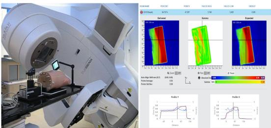
Figure 2: Transit dosimetry assessment of a phantom breast plan on a dynamic platform
