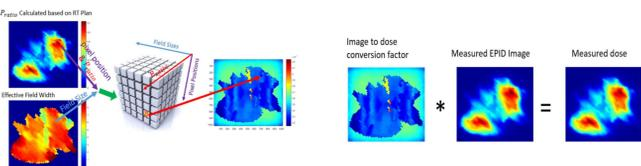
Figure 1: Suncheck calibration process creates a dose conversion matrix for the EPID panel
